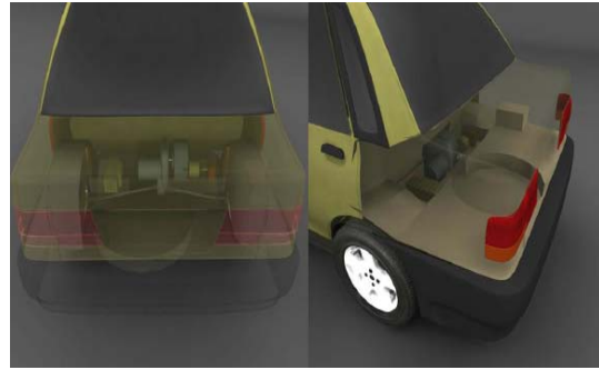
Fig. 4. The schematic of rear-axle in Shaheb 2
