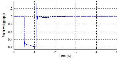
**Fig (23): The 70 KVAR STATCOM Successful Operational Effect on IG Terminal Voltage of Phase 'a' in the FSWT with Longer Fault Duration**
