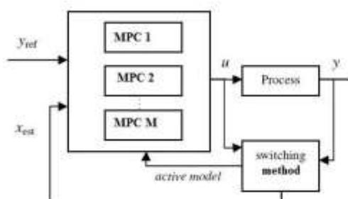
Fig (4): Multiple model predictive control scheme
