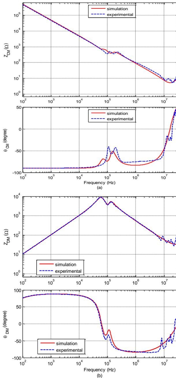
**Fig (8): Comparison between experimental and simulation result for DM and CM: (a)  $Z_{CM}$ , (b)  $Z_{DM}$**
