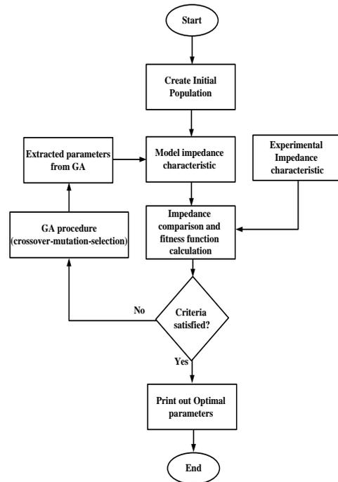
Fig (7): Flowchart of the Genetic Algorithm
