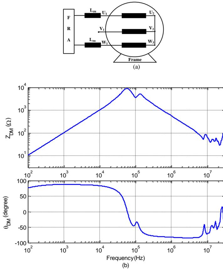
Fig (4): Proposed differential mode configuration ( $Z_{DM}$ ) and its experimental result: (a) Connection diagram (b) Measured impedance (magnitude and phase)
