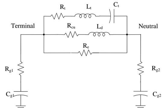
**Fig (1): Proposed per-phase motor winding model**
