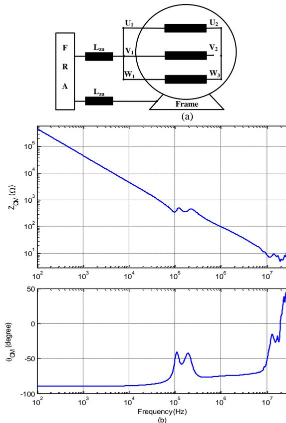
Fig (3): Proposed common mode test configuration ( $Z_{CM}$ ) and its measurement result: (a) Connection diagram (b) Measured impedance (magnitude and phase)
