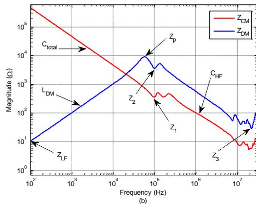
Fig (5): Measured impedances of induction motor
